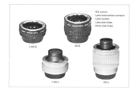
The Pentax Rear Converter A, available in four variations, 1.4X-S\*, 2X-S, 1.4X-L\* and 2X-L, is a new convenient teleconverter accessory, which, when mounted between Pentax 35mm SLR body and any compatible lens, allows 1.4X increase (w/1.4X-S or -L) or doubling (w/2X-S or -L) of the focal length and the set f/number of the master lens in use.
