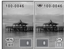
**OK** button The selection frame changes to right image, both images, and left image each time the button is pressed.
