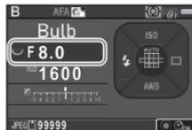
**3** To enable the timed exposure, press **O**, and then use
