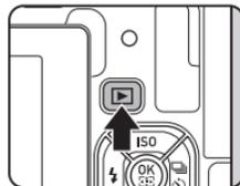
The camera enters playback mode and the most recently captured image is displayed (single image display).
