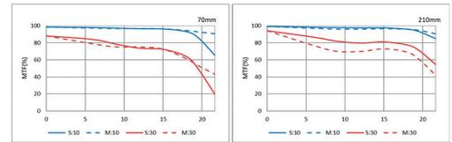
The MTF of high frequency wave (30 lines) possess high level from the center. Especially at the tele side, the high level is maintained till the edge. Also, the MTF of the sagittal and meridional lie aside keeping the level high with less image flow from center to the edge phenomenon.
